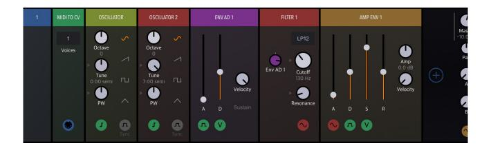
Detune them a bit using the Octave and Tune knobs. You will notice that you hear only Oscillator 2. We don't see green inputs, so nothing is connected to the first Oscillator.
