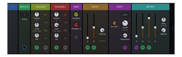
Both oscillators are connected to the mixer. You can control their levels using the corresponding knobs.
