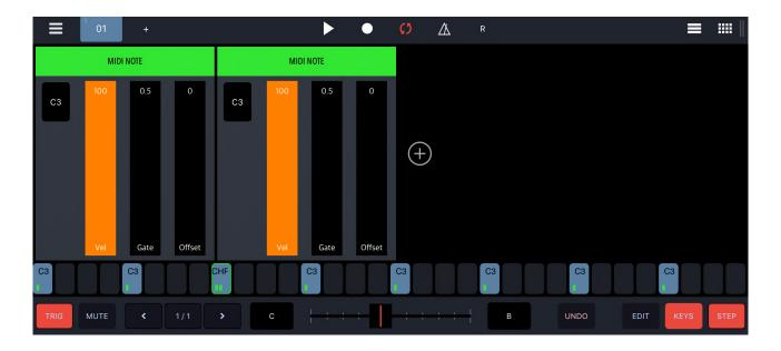
When sequencer reaches a step, all of its components are executed in order, beginning from the left. Conditional component - if condition is not met all succeeding components will not be executed, until next conditional component.
