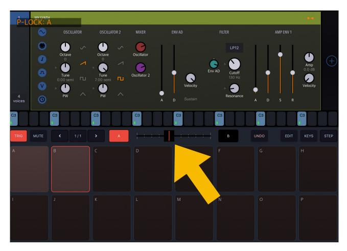
By default you see 2 morph buttons A and B and a morph slider ("crossfader") that morphs between parameters set on A and B state (Linear transition between the values by moving the crossfader).
