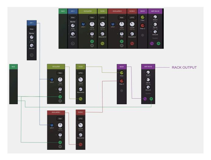
**There are no instant feedback routings in Drambo.** This helps keeping modules well organized and allows you to have up to 8 polyphonic stereo voices in the rack:). You may achieve delayed feedback by using e.g. the Delay rack module or use modules that offer functionality that is commonly achieved by using instant feedback loops.
