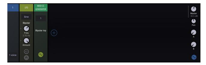
Use the MIDI CC generator module to convert an incoming CV signal to a stream of MIDI CC events. You can select a CC number and configure the input signal type as bipolar or unipolar. (bipolar: -1..1 -> 0..127, unipolar: 0..1 -> 0..127).
